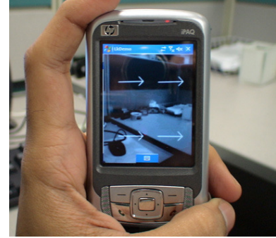
Figure 3: Four sectors of a video frame with their individual motion vectors.
